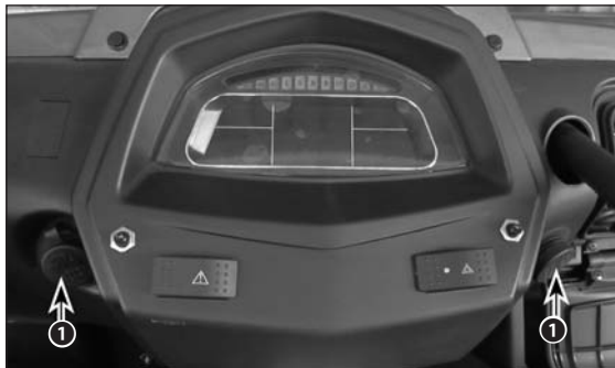
1. 12V DC outlets
